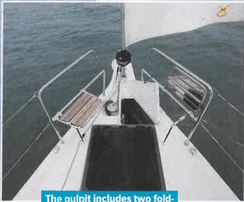
The pulpit includes two fold-down seats; the deep forward locker has ladder access
