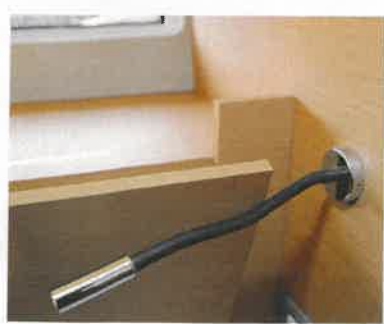
The adjustable reading lights can obstruct the access to large, useful outboard lockers
