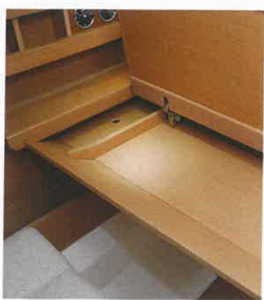
The large chart table would be excellent were it not for the chunky hinges inside
