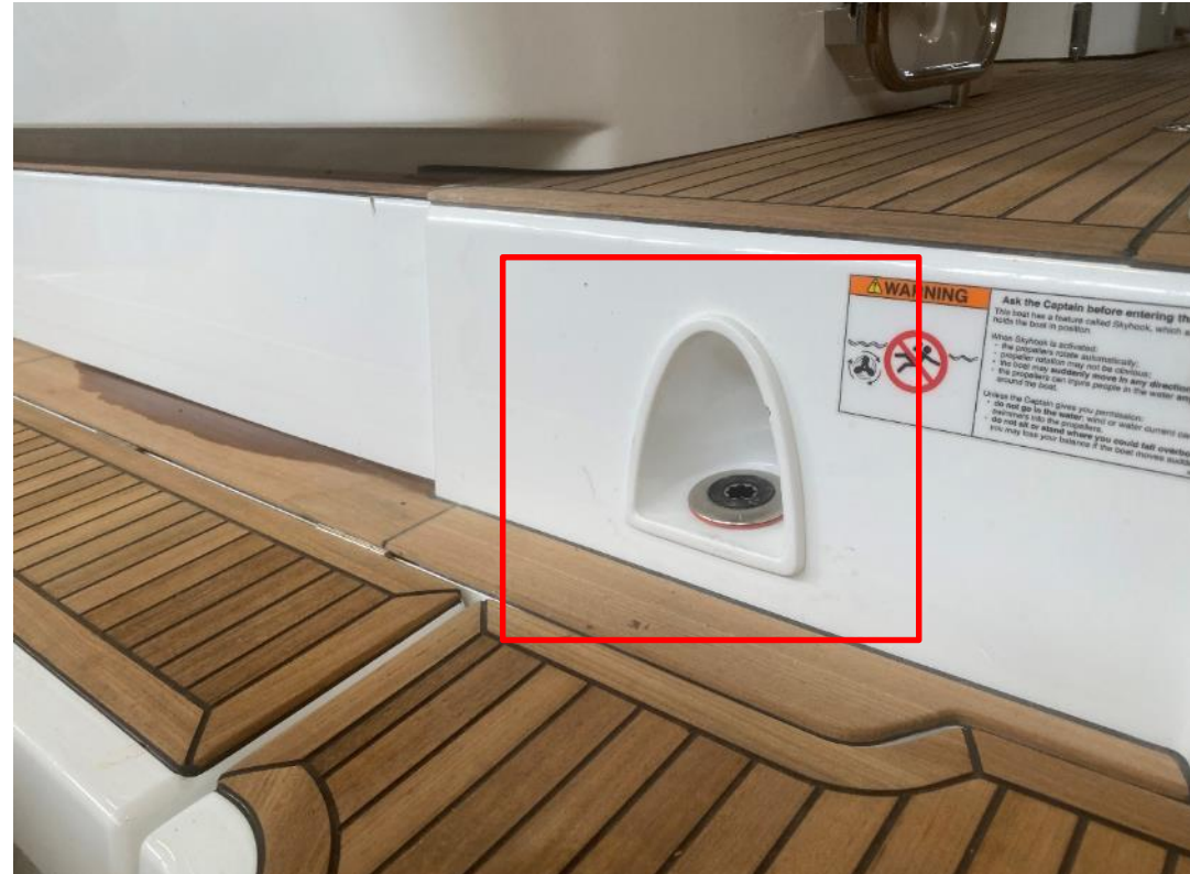
DIESEL TANK FOR GENERATOR
