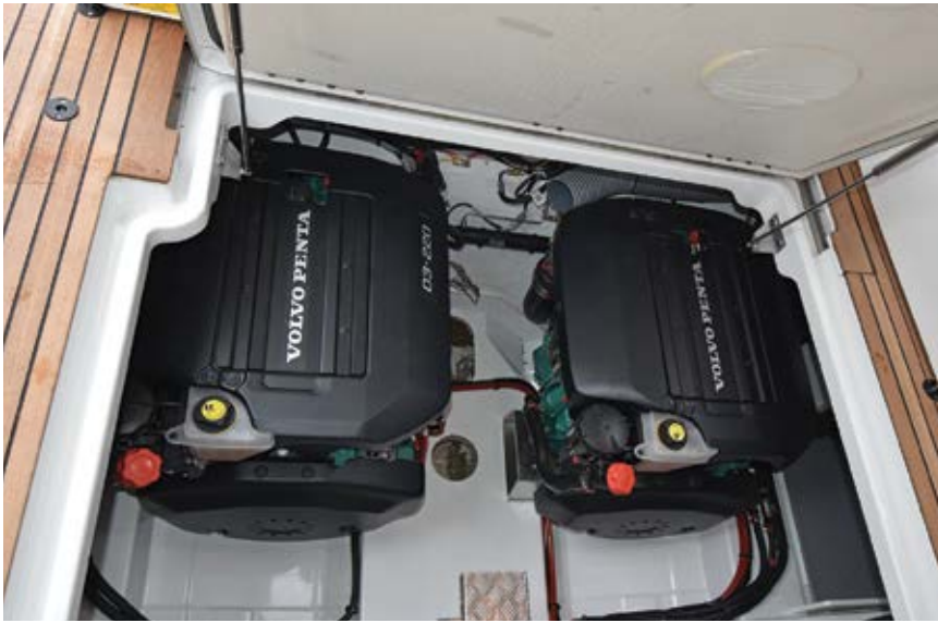
The compact Volvo D3 diesels offer a decent performance and leave plenty of engine bay space
