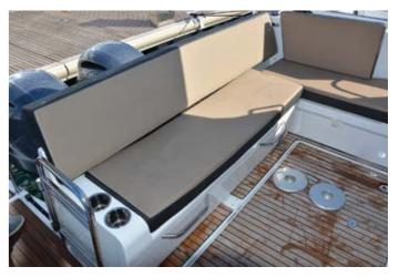
The aft bench slides forwards for engine access
