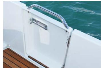
A side access gate in the starboard gunwale is one of the new features found on the 895
